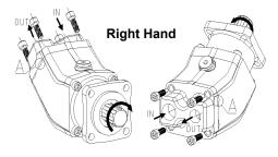
2.3. Screw again the four screws: -torque BI\_M / BI\_M7 = 80Nm -torque BI\_P / BI\_P7 / BI\_H9 = 110Nm
