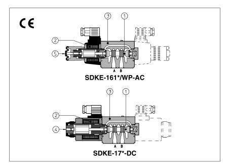
Spool type, two or three position direct operated valves with threaded solenoids.
