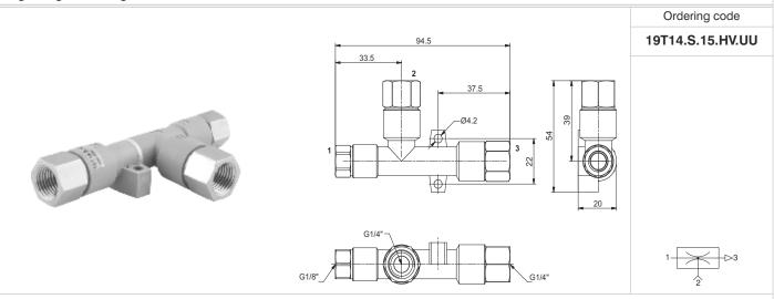
Single-stage generators, robust and reliable, with compact dimensions and suitable for applications which need the required degree of vacuum to be reached quickly with limited air flows. Operating on the Venturi principle, they have the vacuum connection, orthogonal to the axis of supply and outlet. They can be connected directly to the suction cups and/or suction cup holder and applied in any position.
