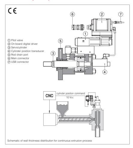
The Parison control is a well known process used in the plastic blow molding machines for the wall thickness distribution of continuous extruded profiles.
