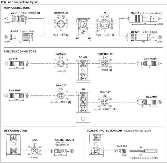
(1) Use of metallic connectors is strongly recommended in order to fulfill EMC requirements
