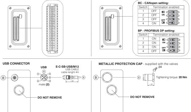
(1) Drivers with BC and BP fieldbus interface are delivered by default 'Not Terminated'. All switches are set OFF (2) Pin layout always referred to driver's view
