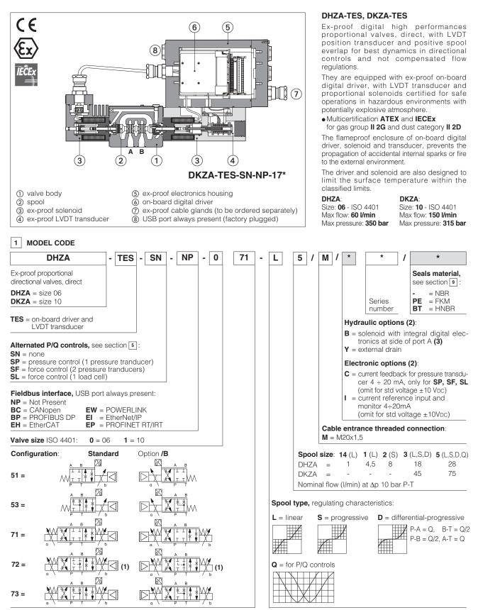
(1) Only for DKZA-\*-S5 the spool overlapping type 2 provides the same characteristic of type 1, but in central position the internal leakages from P to A and B are drained to tank, avoiding the drift of cylinders with differential areas
