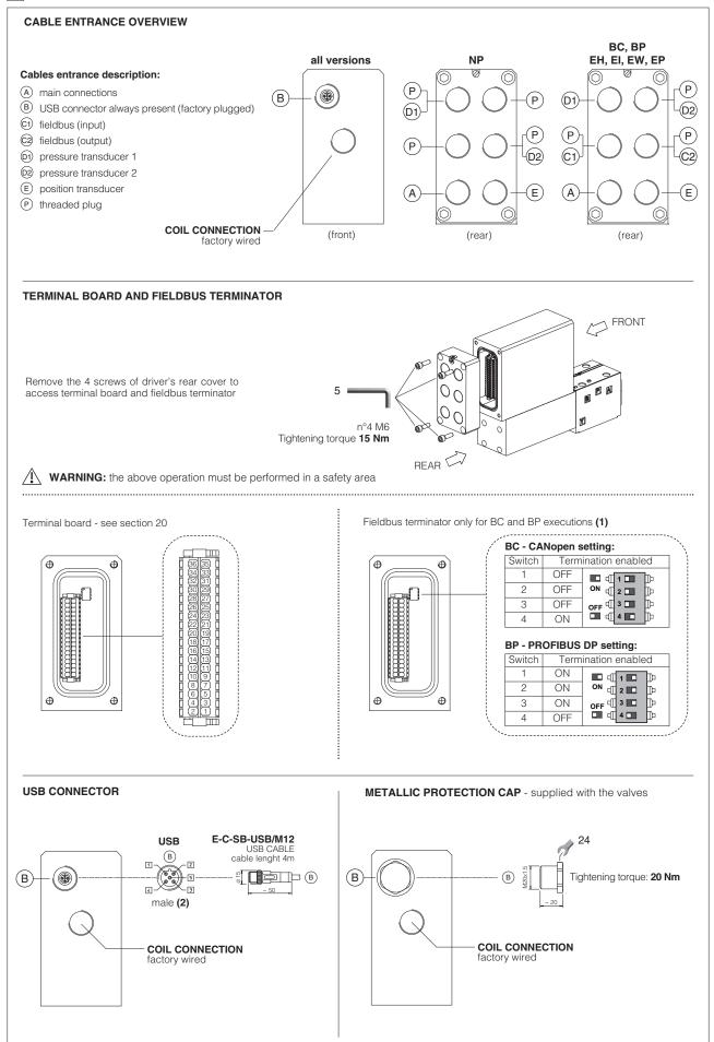
(1) Drivers with BC and BP fieldbus interface are delivered by default 'Not Terminated'. All switches are set OFF (2) Pin layout always referred to driver's view
