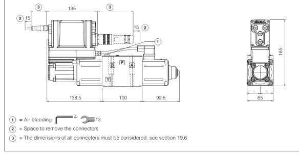
Note: for option /B the proportional solenoid, the LVDT transducer and the on-board digital driver + axis card are at side of port A
