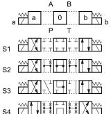
Type **RK**: 2 solenoids - 2 positions with mechanical retention
