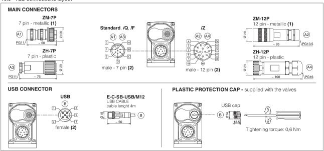
(1) Use of metallic connectors is strongly recommended in order to fulfill EMC requirements
