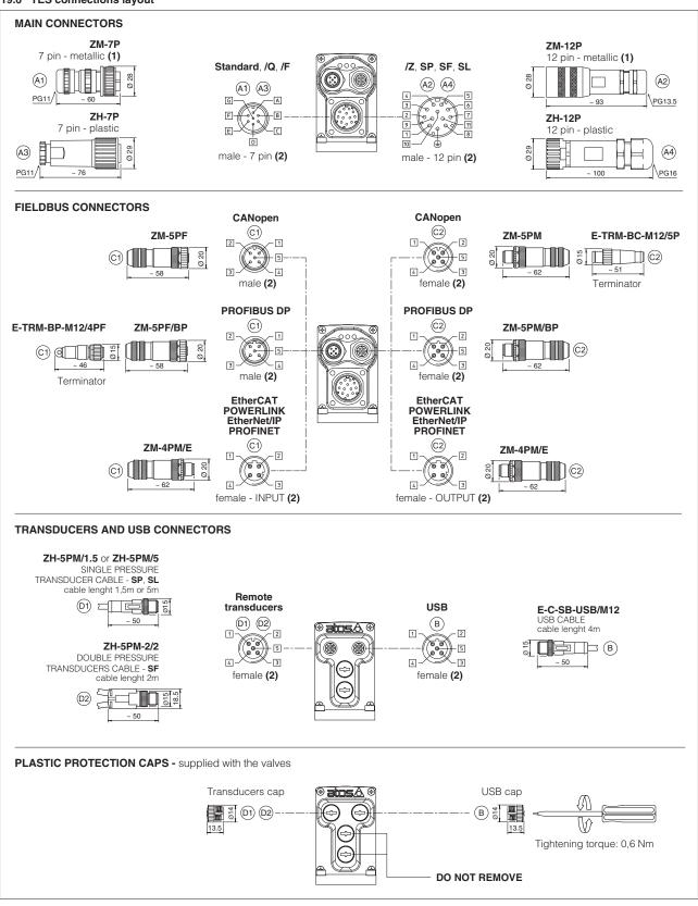
(1) Use of metallic connectors is strongly recommended in order to fulfill EMC requirements (2) Pin layout always referred to driver's view
