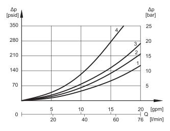
When spool S10 is used for regenerative circuits, pressure drops between A and B lines are described by curve 4.
