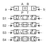
Type **RK**: 2 operations - 2 positions with mechanical retention
