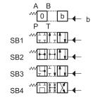
Type **TB**: 1 operation side B 2 external positions with return spring
