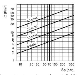
The diagram states the maximum valve controlled flow rate according to the pressure drop between the P and T ports.
