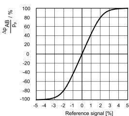
The diagram shows the valve pressure gain, expressed as % of the ratio between the port pressure variation in A or B ( $\Delta p$  AB) and the P system pressure, according to the reference signal. In practice, the pressure gain states the valve reaction towards external disturbances aimed at changing the actuator position.
