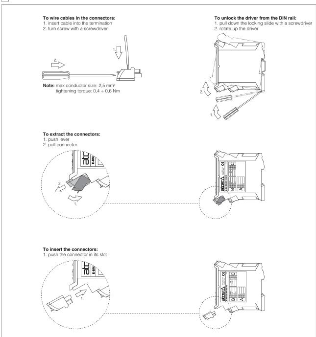
Note: all connectors are supplied with a mechanical coding. This feature ensures a unique insertion of each connector in the own slot (eg. connector A can not be inserted into connector slot of B, C, E, F, G, H)
