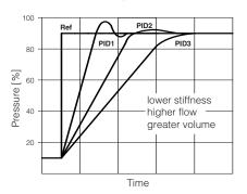
Above indications have to be considered as a general guideline, being affected by hydraulic circuit stiffness, working flow and dead volume. The valve's dynamics can be further optimized on the specific application, customizing PIDs parameters.
