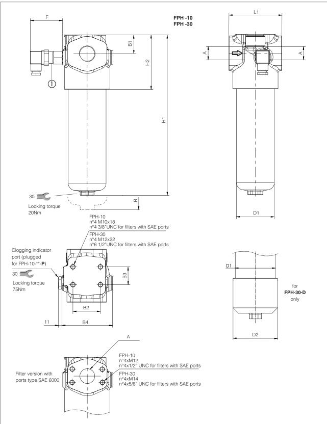
① Optional differential clogging indicator. The drawing shows the electrical indicator type CIA-E\*
