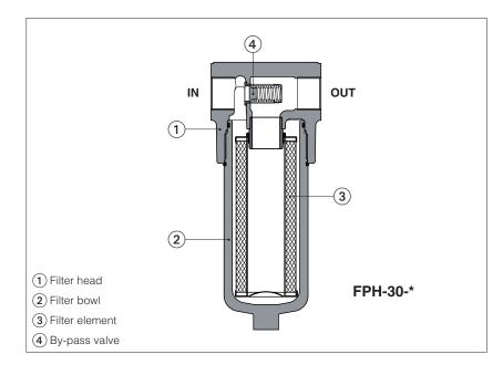
FPH in line filters are designed to protect the whole hydraulic circuit or a single valve from contamination present in the working fluid.
