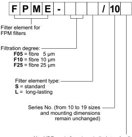
N = NBR seals for mineral oils (standard) V = FPM seals for special fluids (upon request)
