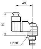
This indicator, apart from giving a visual indication, for example the VPM model, operates by switching an electric contact when the filter element has reached the clogging limit.
