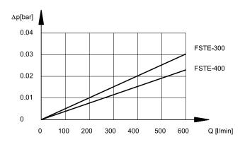
NOTE 2: the filter size has to be selected so that with the nominal flow rate the pressure drop is lower than 0,02 bar.
