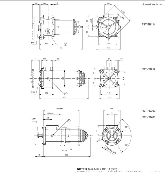
**NOTE 4**: flanges of filters FSU-FS300 and FSU-FS400 are not welded R\* = filter element removal space
