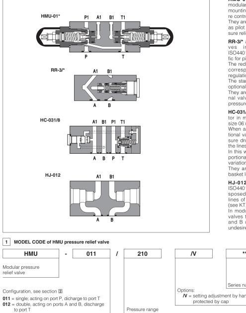
HMU-01 are pressure relief valves in modular execution with ISO4401 size 06 mounting surface, specific for fine pressure control at low flow. They are mainly used for piloting lines and
