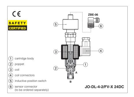
JO-DL are leak free, poppet type solenoid cartridges in screw-in execution normally used to cut off the hydraulic power supply line. They are available in normally closed NC configuration.
