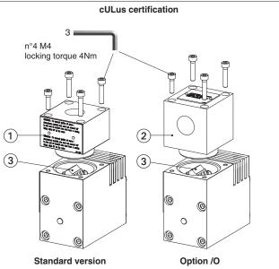
(1) cover with threaded connection for vertical cable gland fitting 2 cover with threaded connection for horizontal cable gland fitting ③ terminal board for cables wiring
