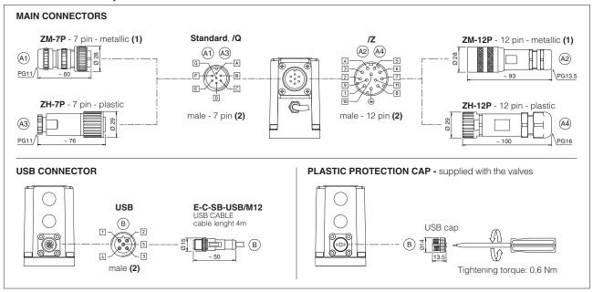
(1) Use of metallic connectors is strongly recommended in order to fulfill EMC requirements
