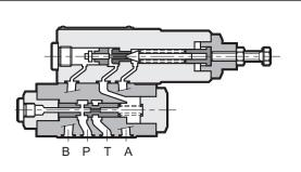
— MRQA is a pressure relief and safety valve with automatic unloading. Upon reaching the set value, the valve freely unloads the pump and puts it under pressure again when the pressure values descend in the circuit to correspond to 63% or 75% of the set value.
