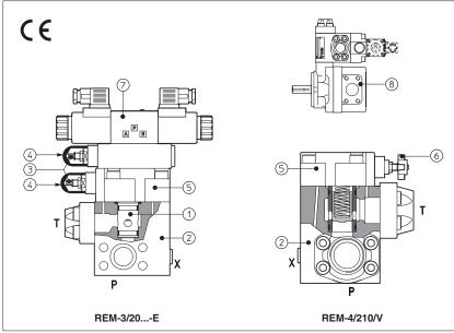
**REM** are two stage pressure relief valves with balanced poppet and SAE flange connection, designed to operate in oil hydraulic systems.
