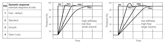
Above indications have to be considered as a general guideline, being affected by hydraulic circuit stiffness, working flow and dead volume. The valve's dynamics can be further optimized on the specific application, customizing PIDs parameters.
