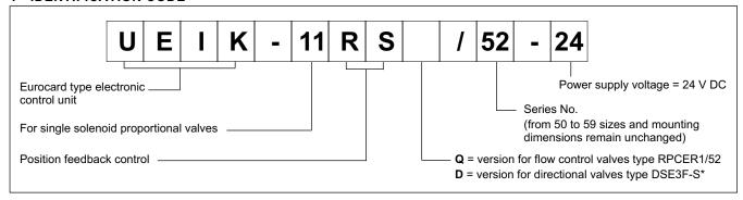
The UEIK-11RS\*/52 card is an electronic control unit Eurocard type for closed loop control of single solenoid proportional valves with positional feedback control.
