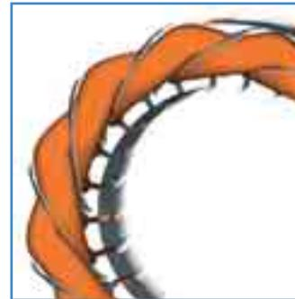
The copper is impregnated with a double layer of H class insulating enamel to ensure high resistance to electrical, thermal and mechanical stress. The phases are further isolated by another layer of Nomex film to protect the motors from the voltage peaks that usually occur when the motor is controlled by an inverter.
