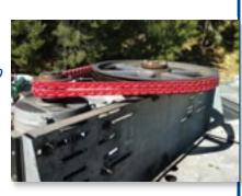
Solution On upgrading to PowerTwist Plus V-Belts, the maintenance team now carries boxes of the red belt 24/7. Drives are now serviced quickly without wasting time returning to the belt crib to pick up specific belt sizes. Stock was reduced to just a few boxes of 3L, A/13 and B/17 sections.
