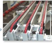
designing with PowerTwist Friction Top from the start, they were able to produce systems that rarely require maintenance to the belts, but can be done in minutes if the need does arise.
