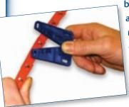
belt off, take out a link and roll it back on no need to move any drive components. No time — no trouble.
