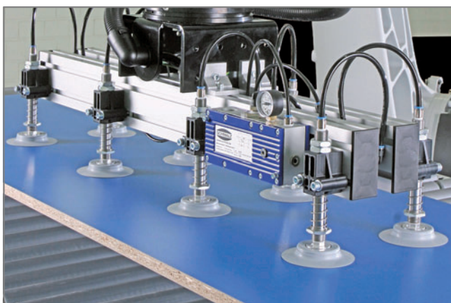
Suction plates SPU being used for handling coated chipboards
