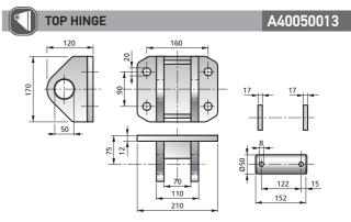
It is recommended the fitment of two spacers ensuring the top bearing to be centered on the support and to swivel properly (+/-7°). These spacers are included.
