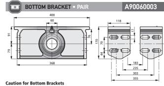
Recommended backlash between pin over-bosses and brackets / supports = 3 mm total (1.5 mm each side). It is recommended to fit M16 bolts/nuts, type 8.8 or better.
