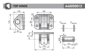
**Caution for Top Hinge**It is recommended the fitment of two spacers ensuring the top bearing to be centered on the support and to swivel properly (+/-7°). These spacers are included.
