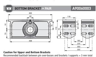
(1.5 mm each side). It is recommended to fit M16 bolts/nuts, type 8.8 or better.
