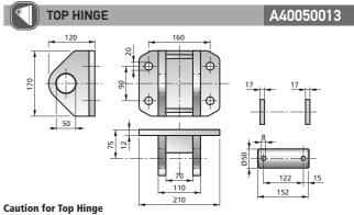
It is recommended the fitment of two spacers ensuring the top bearing to be centered on the support and to swivel properly  $(+/-7^{\circ})$ . These spacers are included.
