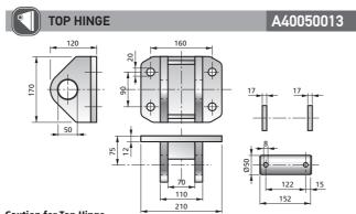
**Caution for Top Hinge** It is recommended the fitment of two spacers ensuring the top bearing to be centered on the support and to swivel properly  $(+/-7^\circ)$ . These spacers are included.
