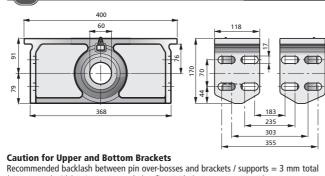
(1.5 mm each side). It is recommended to fit M16 bolts/nuts, type 8.8 or better.
