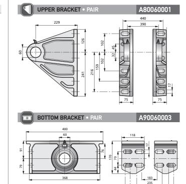
**Caution for Upper and Bottom Brackets** Recommended backlash between pin over-bosses and brackets / supports = 3 mm total (1.5 mm each side). It is recommended to fit M16 bolts/nuts, type 8.8 or better.
