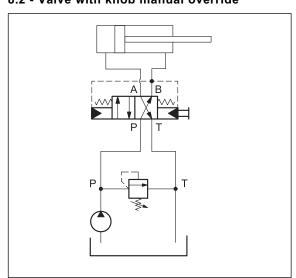
To set the system relief valve correctly, the self-reversing function must be inactive.
