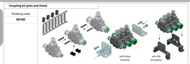
Weight 2,5 gr. - The kit, which includes a series of pins and forks, enables to join together in a fast and safe way the function fittings. The pins, once inserted in the front holes, ensure resistance against forces applied perpendicularly and sideway (for example the insertion of the tube in the cartridges). The forks, once located in the profiled housing ensures that the parts are held together tightly. The kit allows for 5 function fittings to be mounted together.
