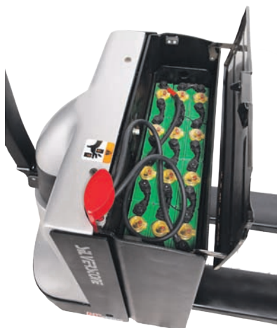
Central water filling system
