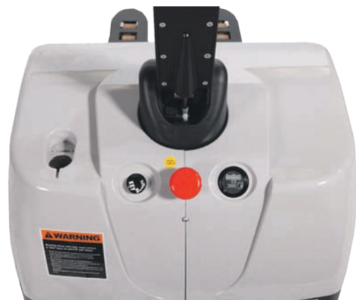
Curtis controller with battery indicator
