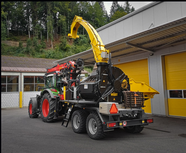
SMC-610 PT0-T with hydraulic accelerator and folded-down maintenance platform.
