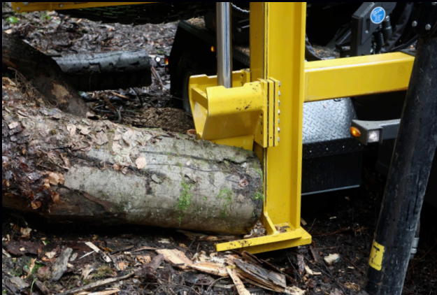
Type: Wüst, pressure: 50t, split-height: 1150mm
